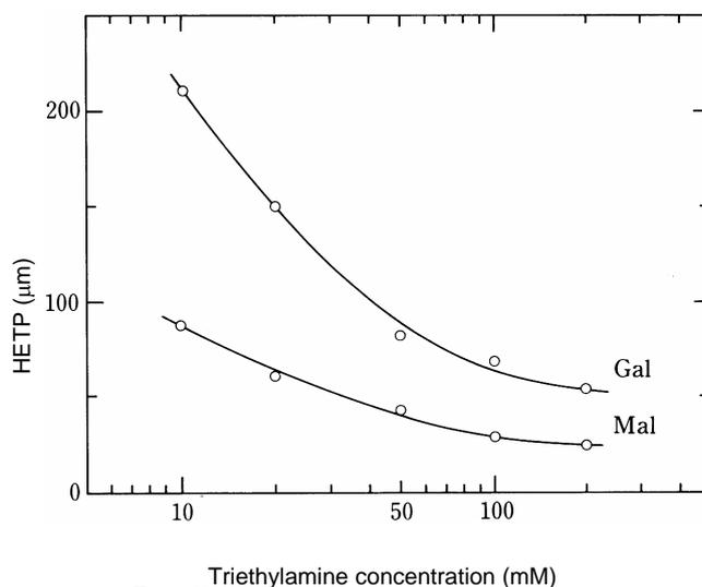
Figure-7 Effect of concentration of triethylamine added to mobile phase on HETP
