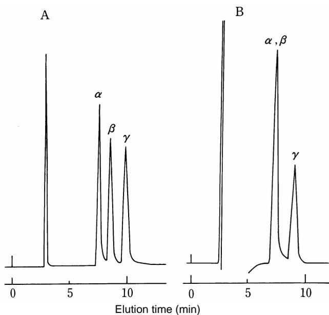
**Figure-5 Separation of  $\alpha$ ,  $\beta$ ,  $\gamma$ -cyclodextrins**
