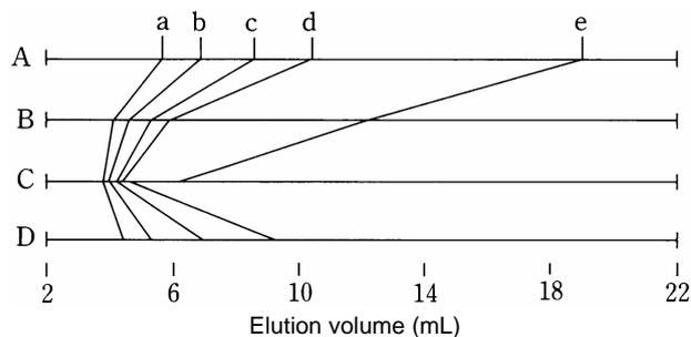
**Figure-3 Changes in eluent composition and polyol retention volume on TSKgel Amide-80**
