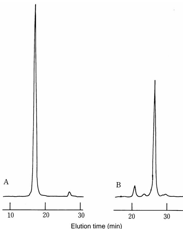
**Figure-10 Analysis of pyridylaminated derivative of oligosaccharide on TSKgel ODS-80TM and TSKgel Amide-80**
