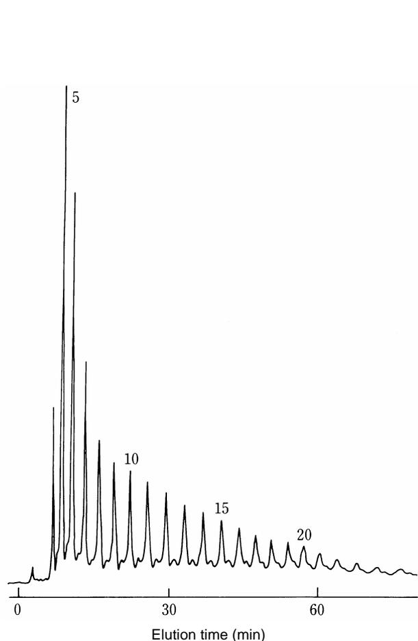
**Figure-9 Separation of pyridylaminated derivative of dextran hydrolysate**
